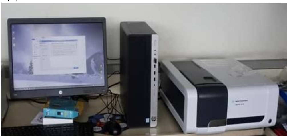
A newly procured HPLC Equipment used by Food Security Subprogramme Researchers for separation and qualification of amino acid in banana and quantifying sugar and acids on juice
